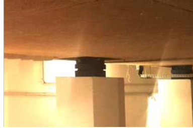
Figure 17: Example of the elastic supports of the chambers of the acoustic laboratory.
