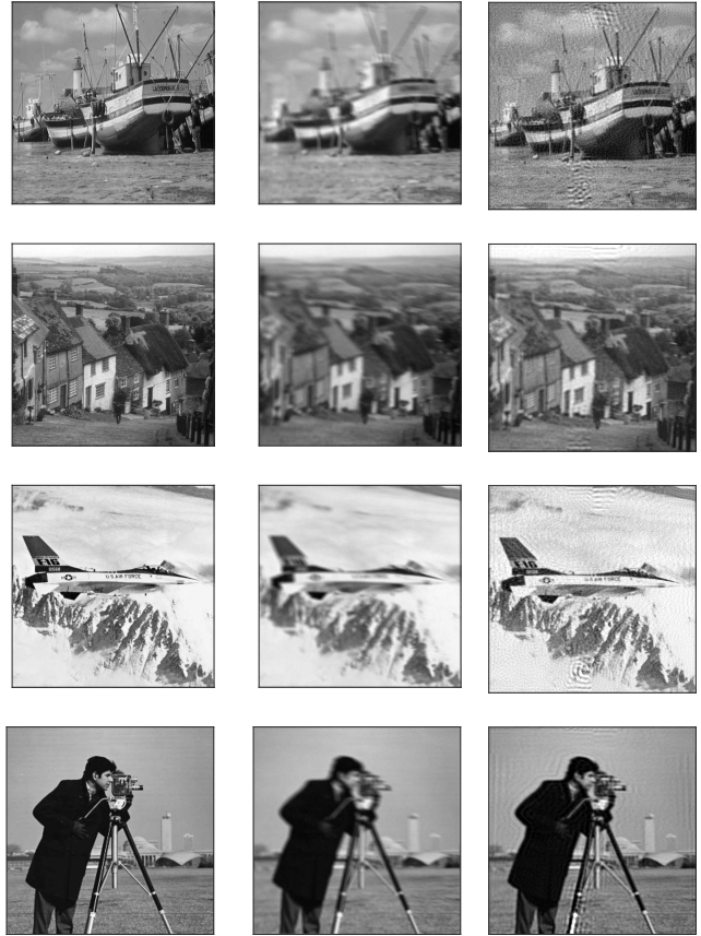
Fig. 14. (left) Original images ; (middle) blurry noisy versions with \sigma_n = 0.01 ; (right) example of restored image using the mean blur estimate from one run of GIANPF.
