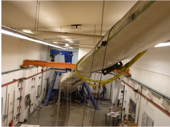
Figure 3. Experimental setup of the SSP 34 meters wind turbine blade manufactured by SSP-Technology A/S. The blade was instrumented with 10 accelerometers along the leading edge (LE) and 10 along the trailing edge (TE) and was excited by an electromechanical actuator. The debonding damage was introduced into the blade (García and Tcherniak 2019).
