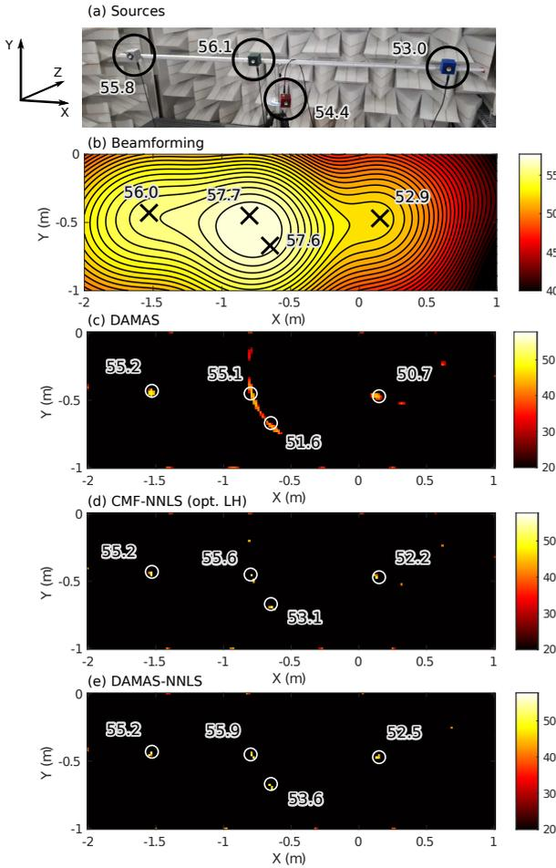
Figure 2: 2D experiment,  $F = 1806$  Hz. Comparison of (a) actual powers of the sources, (b) beamforming, (c) DAMAS, (d) CMF-NNLS, and (e) DAMAS-NNLS. Powers in dB. Actual positions are indicated by crosses in (b), circles in (c) (d) and (e). Numbers indicate the power summed in the circles of radius 0.05m around the true locations of the sources.
