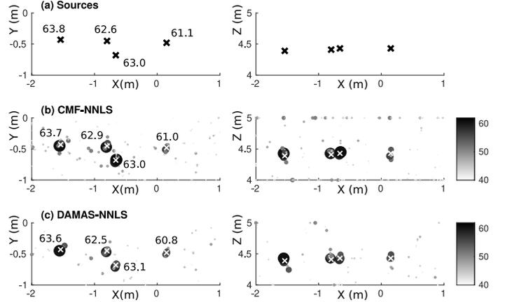
Figure 4: 3D experiment,  $F = 4858$  Hz. Front (left) and top (right) view. (a) Positions and powers of the sources. Results of (b) CMF-NNLS and (c) DAMAS-NNLS. Estimated powers and positions of the sources are indicated by discs with radius proportional to the power, actual positions by crosses. Indicated powers in dB are obtained by summing the estimated powers in a sphere of radius  $R = 0.08$ m around the actual position of the sources.
