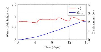
Fig. 8. The Super-Sauze landslide data from the literature: Displacement measurement  $d_{mea}^k$  and water table height time-series  $w_t^k$  (Bernardie et al., 2014)
