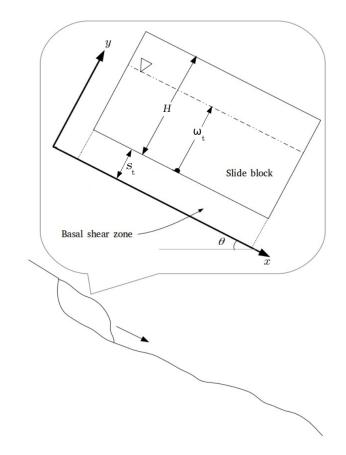
Fig. 1. Geometrical variables of the slide block
