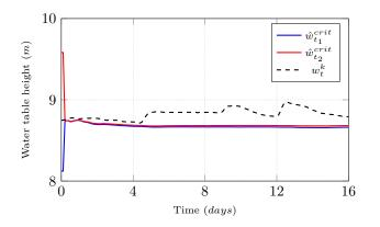
Fig. 13. Time evolution of parameter estimate  $\hat{w}_{t_1}^{crit}$  ( $\rho=1700~kg/m^3), \hat{w}_{t_2}^{crit}$  ( $\rho=2140~kg/m^3)$  and  $w_t^k$
