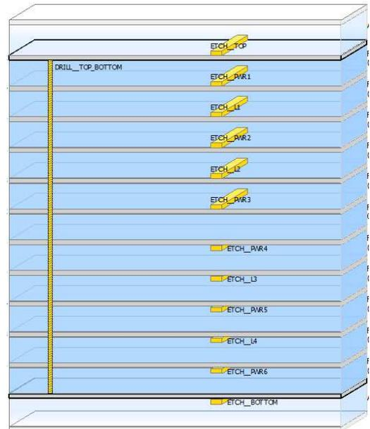
*Fig. 2.* Cross section of the case study
