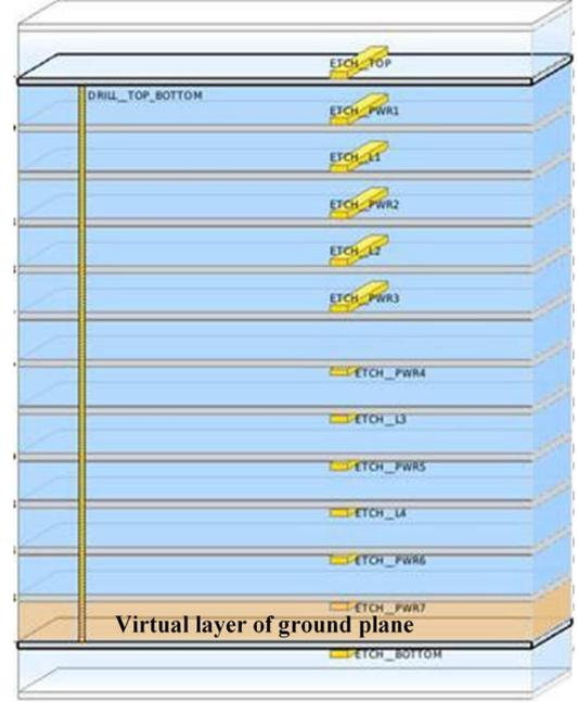
Fig. 7. Cross section of the modified design
