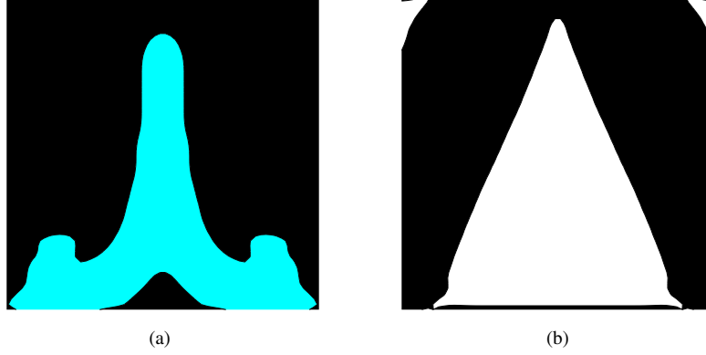
Figure 10: Optimal topology for \bar{F}_{2221} : (a) PZT/polymer; (b) PZT/void.
