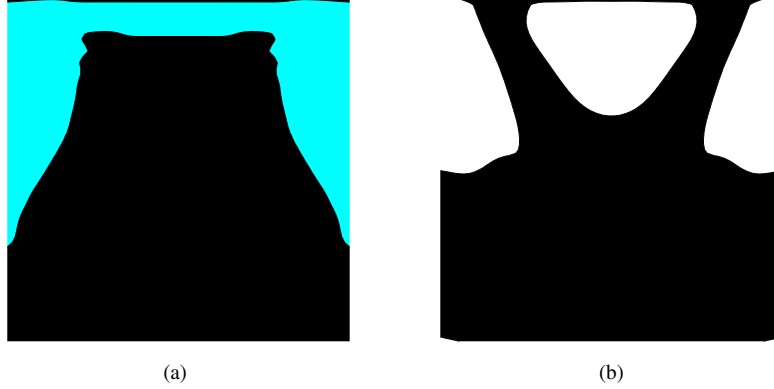
Figure 11: Optimal topology for \bar{F}_{1112} : (a) PZT/polymer; (b) PZT/void.
