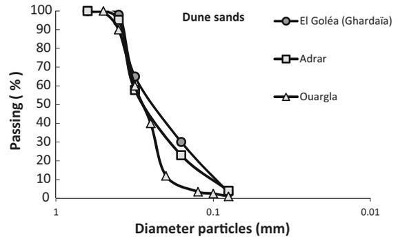
**Fig. 3** Particle size distribution curves of dune sands (Adrar–El Goléa–Ouargla)
