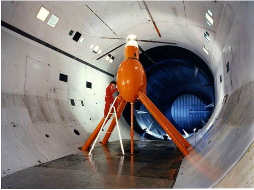
Figure 1: 7A rotor in ONERA Modane S1MA Wind Tunnel.
