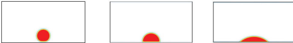
(a) \frac{\rho^s}{\rho^l} = 0.05 \theta = 140.67^\circ (b) \frac{\rho^s}{\rho^l} = 0.3 \theta = 86.19^\circ (c) \frac{\rho^s}{\rho^l} = 0.6 \theta = 52.26^\circ
