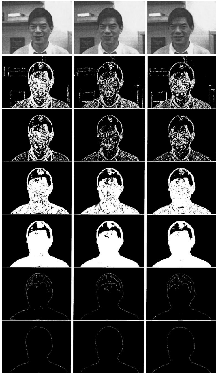
Fig. 3. 1st row: Original active video sequence (frame 10, 24, 41); 2nd row: Compensated frame differences; 3rd row: Noise remove using morphological filtering ( kernel = 9 \times 9 ); 4th row: Consecutive frames fusion; 5th row: Motion areas detected by smoothed fusion frames (closing); 6th row: Contours of motion areas; 7th row: Detected silhouette of the motion head.
