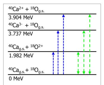
**FIGURE 5** | Coupling scheme adopted in the DWBA (blue dotted single arrows) and CC (green dashed double arrows) calculations in the present work. In DWBA, the single arrows sketch that back coupling effects are not included.
