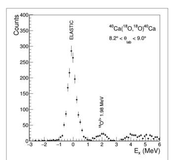
**FIGURE 1** | Excitation energy spectrum of  $^{40}$ Ca obtained in the  $^{18}$ O +  $^{40}$ Ca elastic scattering and inelastic scattering at an incident energy of 275 MeV and  $8.2^{\circ} < \theta_{lab} < 9.0^{\circ}$ .
