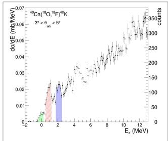
**FIGURE 3** | Excitation energy spectrum of the  $^{40}$ Ca( $^{18}$ O,  $^{18}$ F) $^{40}$ K charge exchange reaction at 275 MeV and 3° <  $\theta_{lab}$  < 5°. The three hatched areas indicate the regions of interest for the study of the angular distributions.
