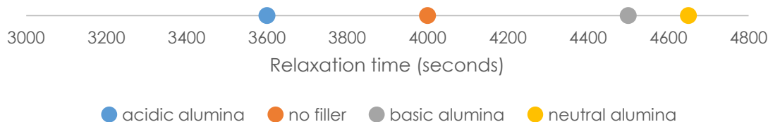
13 Figure 4. Effect of different functionalization of alumina fillers on vinylogous urethane vitrimer composites relaxation time.
