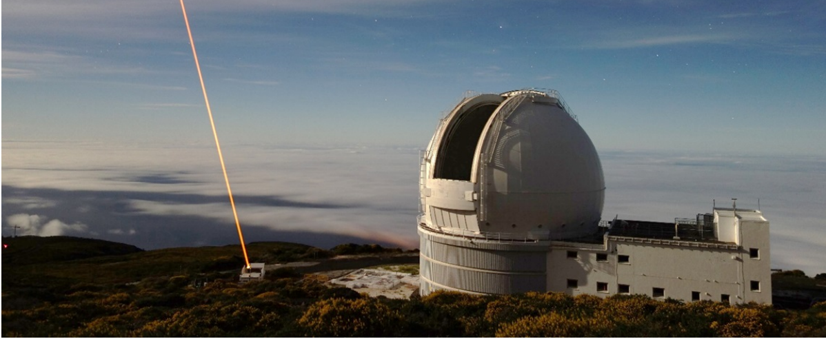
Figure 3. 'Wendelstein' Laser Guide Star Unit and William Herschel Telescope
