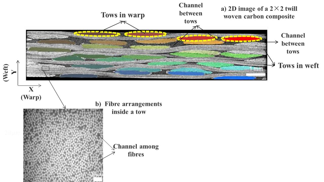
Fig. 1: The schematics of the dual porosity: (a) a 2/2twill woven carbon composite cross section, orthogonal to the warp (channels between tows forming inter-tow porosity), (b) Fibres inside a tow (channels between the fibres forming intra-tow porosity) the images with permission from [6].
