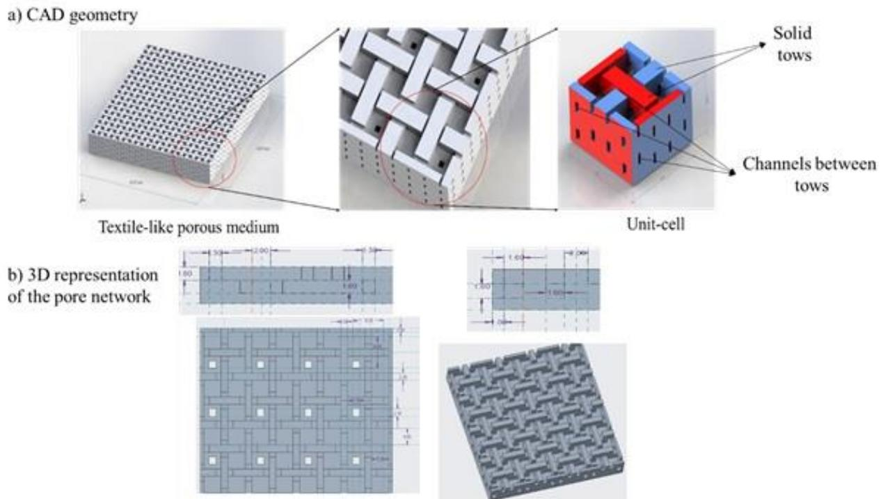
Fig. 3: The schematic of the textile-like porous medium: (a) A CAD geometry of the textile-like porous medium (top). (b) The dimension of the textile-like porous medium (below)
