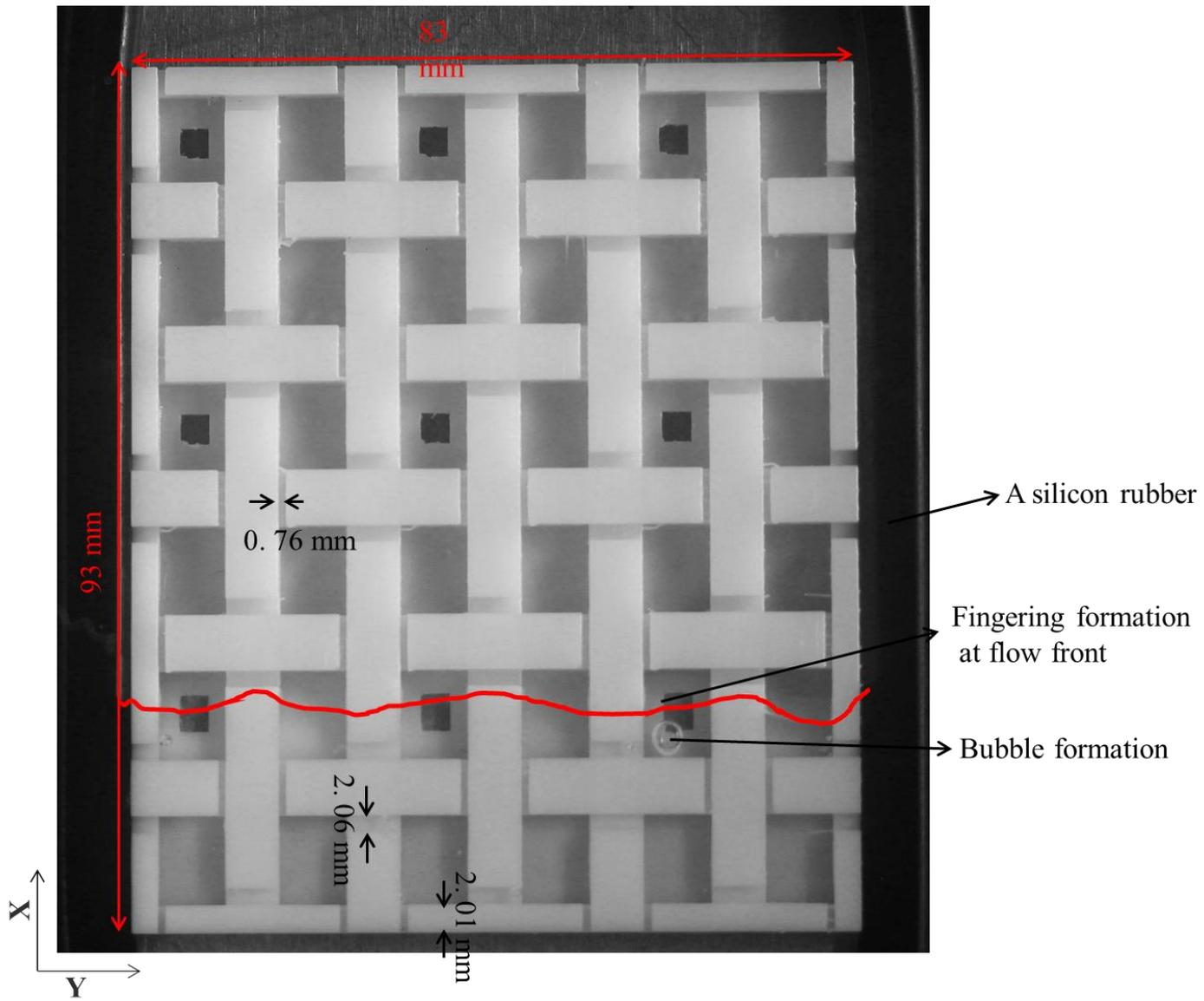
Fig.5: The flow front pattern during the impregnation process
