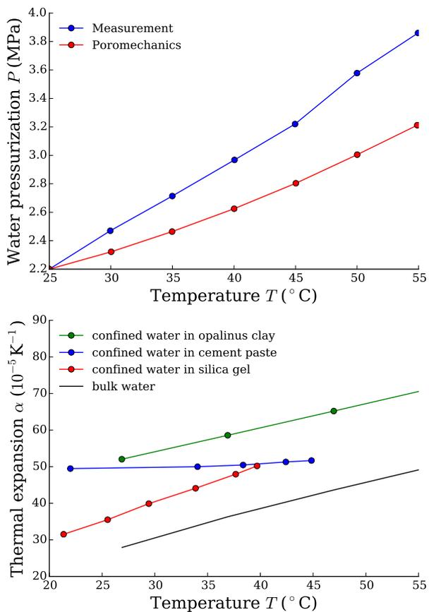
**Fig. 1** (top) Interstitial water pressurization in Opalinus Clay during an undrained heating experiments and compared to the prediction with usual poromechanics assuming bulk properties for water (adapted from [26]). (bottom) Experimental results showing the anomalous thermal expansion of confined water (adapted from [26] with data from [40] and [16]).
