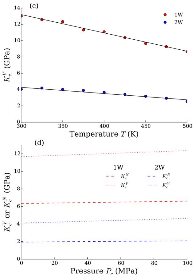
**Fig. 6** Undrained rigidities of confined water in Na-Montmorillonite. (top) Evolution of  $K_c^V$  with temperature. (bottom) Evolution of  $K_c^V$  and  $K_c^N$  with confined pressure for 1W and 2W waters.
