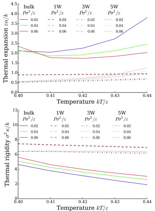
**Fig. 5** Thermal expansion (top) and thermal rigidity (bottom) isobars of the LJ fluid bulk and confined in the slit pore. The results are reduced with respect to the LJ parameters  $\sigma$  and  $\epsilon$ .
