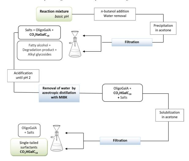
Figure 5. Procedure based on successive filtrations for the isolation of purified *n*-oleyl D-galactosiduronic acids  $CO_2HGalC_{18}$ .
