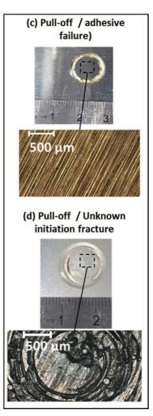
Fig. 4. (A) Pictures of the adhesive fracture initiation by Single Lap Joint test; (B) Picture of adhesive fracture initiation after Three-Point bending test; (C) Picture of adhesive initiation after pull-off test; (D) Picture of an unknown initiation fracture after pull-
