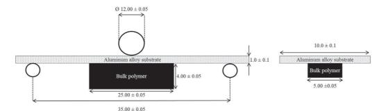
and tested for each configuration. This test was performed with a tensile machine (INSTRON 3369, Élancourt, France), fitted with a 500 N full-scale load cell with a sensitivity of 0.5% of the measured values and was carried out at room temperature (23 °C  $\pm$  2 °C). The displacement rate was 0.500  $\pm$  0.003 mm min $^{-1}$  in the Three-Point configuration (see Fig. 3). The ultimate load, FMax, was considered as the failure initiation measurement.
