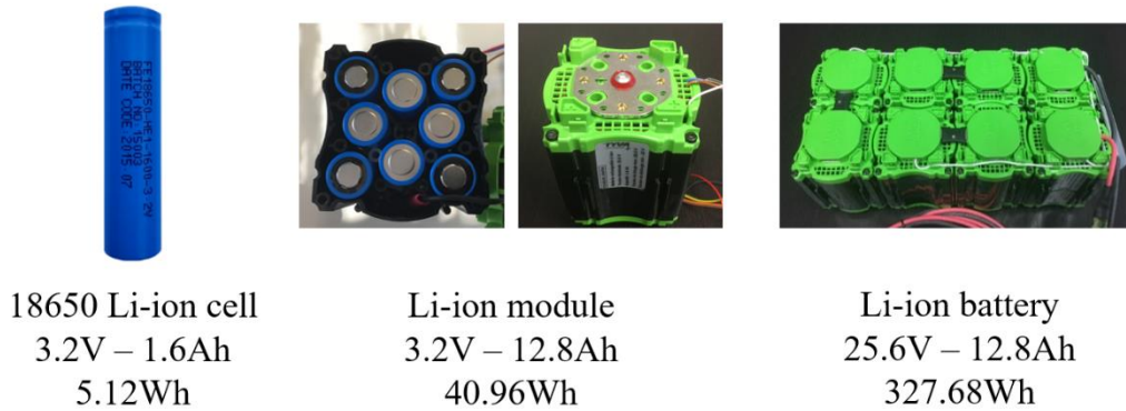
Fig. 3 LiFePO 4 /graphite Li-ion cell, module and battery developed by TYVA ENERGY.
