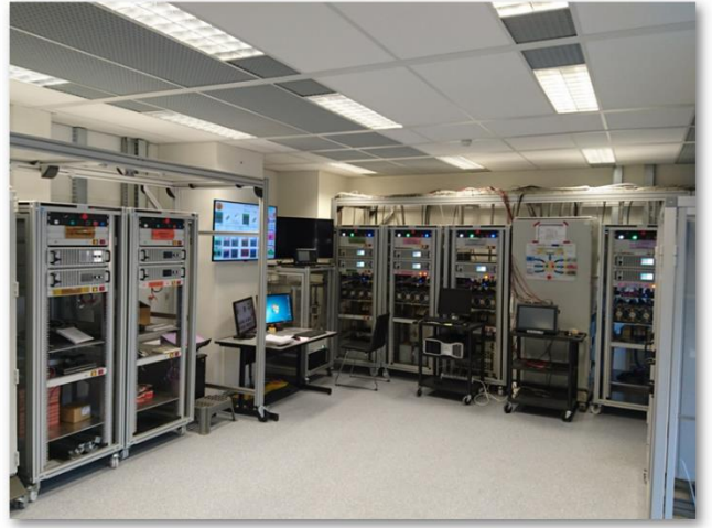
Fig. 1 Concept of the battery emulator (left) and test bench for power HIL simulation experiments (right).
