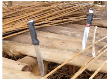
Various knives used to cut and sharpen the reeds
