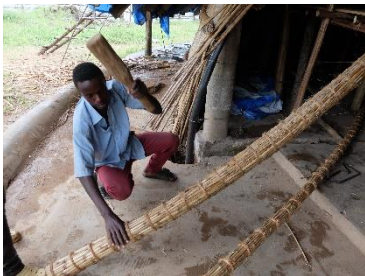
Curving a ring with the wooden mallet
