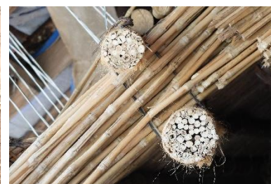
Cutting single reeds and full rings with the hacksaw. The picture on the right shows the neat cut obtained.
