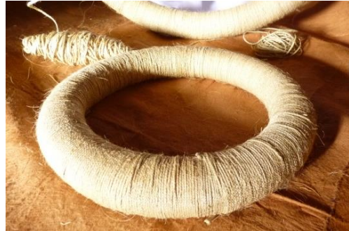
The ring is then wrapped with hand-braided sisal rope
