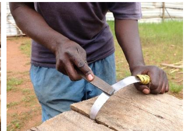
Blade sharpening with a file
