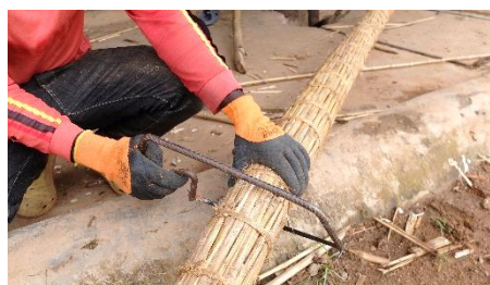
Cutting single reeds and full rings with the hacksaw. The picture on the right shows the neat cut obtained.
