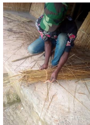
Combing a bundle with a stick to remove unwanted elements and tying the bundle in a conical shape with a sisal rope 4 photos by Brian Kalema
