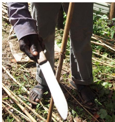
Smoothing the reeds with a knife
