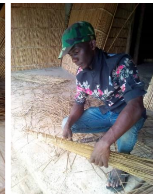
Combing a bundle with a stick to remove unwanted elements and tying the bundle in a conical shape with a sisal rope 4 photos by Brian Kalema
