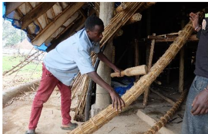
Curving a ring with the wooden mallet
