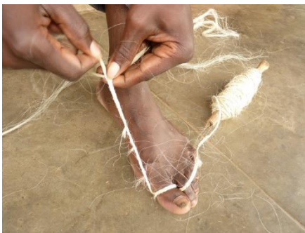
Braiding the sisal rope used to wrap the rings
