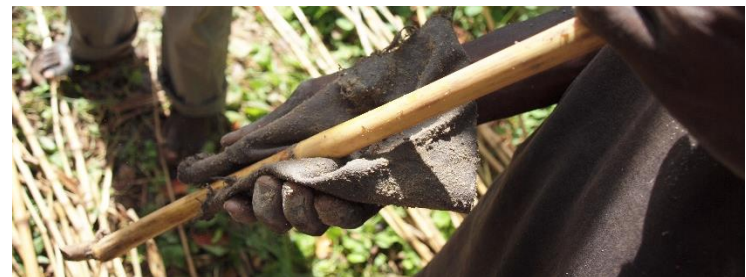
Smoothering reeds with a rag filled with sand
