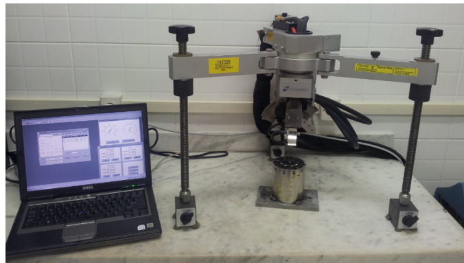
Figure 3. X-ray residual stress analyzer.
