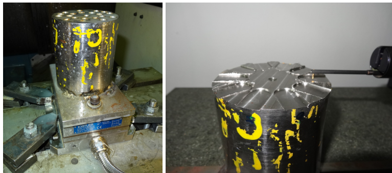
(a) Dynamometer and work-piece.
