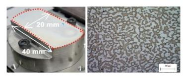
(a) Workpiece material (b) Microstructure **Figure 2.** Super duplex stainless steel (UNS S 32750)
