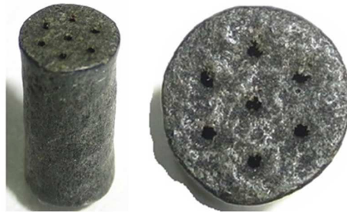
Figure 1. Pictures of propellant P1 mainly composed of nitrocellulose.
