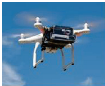
Figure 13. GNSS/RTK receiver mounted on a DJI Phantom 3
