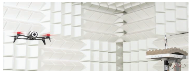
Figure 8. UAV flying in the ISL anechoic chamber (rotating device for the microphonic array on the right)
