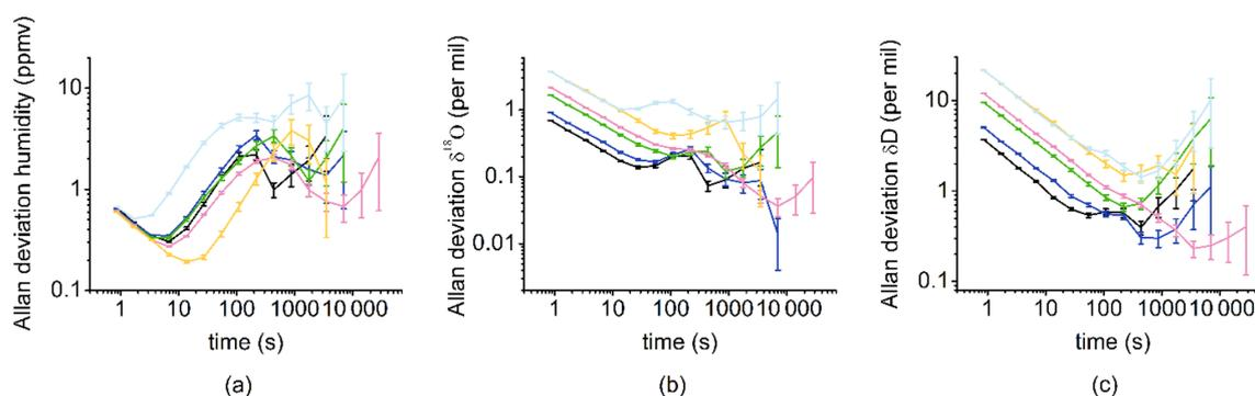
**Figure 3.** Allan deviation over 4 h for different humidity levels (black, 1080 ppmv; dark blue, 770 ppmv; green, 400 ppmv; pink, 320 ppmv; yellow and light blue, 170 ppmv) for humidity (a),  $\delta^{18}\text{O}$  (b) and  $\delta\text{D}$  (c).
