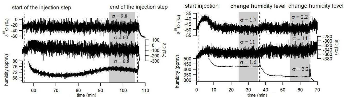
**Figure 4.** Records of  $\delta^{18}\text{O}$ ,  $\delta\text{D}$  and humidity over three humidity plateaus (72 ppmv on the left, 425 and 335 ppmv on the right) obtained with the LHLG. The gray rectangles indicate the period (10 min) over which the average values are kept for calibrating the data generated by the L2130-i analyzer.**Table 3.** Set points for the water infusion rate and dry-air flow at a temperature of 20 °C.
