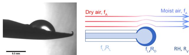
**Figure 1.** Evaporation of a droplet in the humidity generator chamber: the left panel shows a picture from the prototype from Landsberg (2014), and the right panel displays schematics of the water molecules being transferred to the air flow (Casado, 2016).
