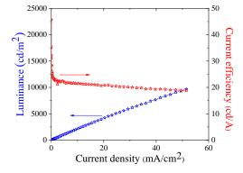
**Figure 7.** Left. ORTEP (50 % ellipsoid probability) of **2,7-DiCbz-SBF-4'-POPh**<sub>2</sub>. Right. Luminance and current efficiency as a function of current density for the SL-PhOLED D48 (ITO/PEDOT:PSS/**2,7-DiCbz-SBF-4'-POPh**<sub>2</sub>:**Ir(ppy)**<sub>3</sub>(10 %) /LiF/Al).
