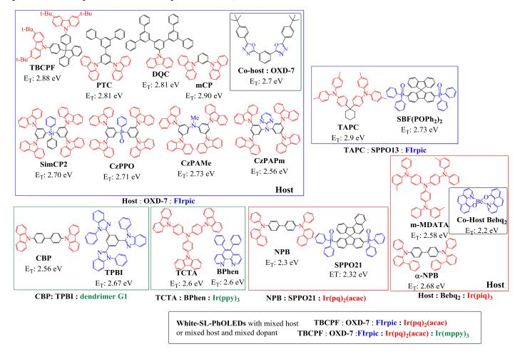
**Figure 14.** Molecular structure of hosts and co-hosts used in SL-PhOLEDs with mixed-hosts in EML. In the host materials, black, blue and red fragments respectively point the  $\pi$ -linker, the acceptor and the donor units of the OSC.
