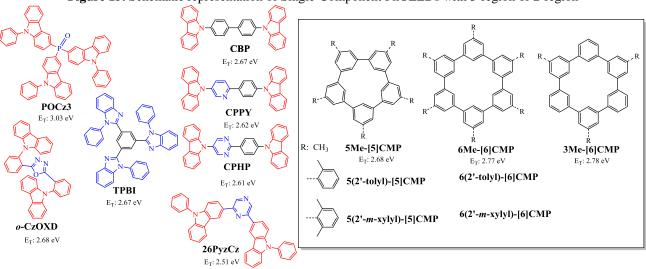
**Figure 16.** Molecular structure of host materials used in single-component PhOLEDs. In the host materials, black, blue and red fragments respectively point the  $\pi$ -linker, the acceptor and the donor units.
