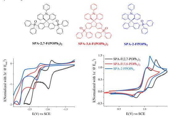
**Figure 4.** Normalized cyclic voltammograms of  $SPA-2,7-F(POPh_2)_2$  (black lines),  $SPA-3,6-F(POPh_2)_2$  (red lines) and  $SPA-2-FPOPh_2$  (blue lines) in the cathodic (left, DMF + BuN<sub>4</sub>PF<sub>6</sub> 0.1 M) or the anodic (right,  $CH_2Cl_2 + Bu_4NPF_6$  0.2 M) range. Sweep-rate: 100 mV.s<sup>-1</sup>, platinum disk working electrode.
