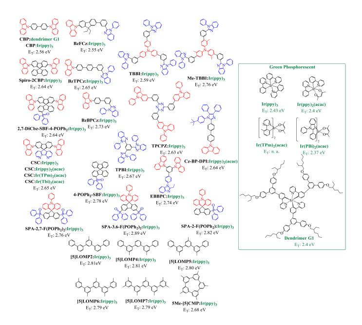
**Figure 6.** Molecular structure of host materials and green phosphors used in green SL-PhOLEDs.  $E_T$  in black (green) is that of the host (phosphorescent emitter). In the host materials, black, blue and red fragments respectively point the  $\pi$ -linker, the acceptor and the donor units of the OSC.
