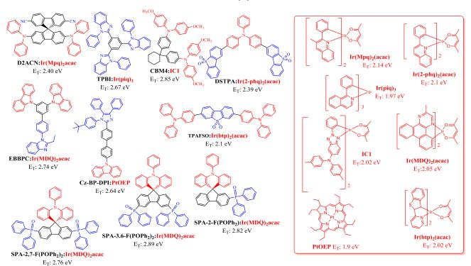
**Figure 9.** Molecular structure of host materials and red phosphors used in red SL-PhOLEDs  $E_T$  in black (red) is that of the host (phosphorescent emitter). In the host materials, black, blue and red fragments respectively point the  $\pi$ -linker, the acceptor and the donor units of the OSC.
