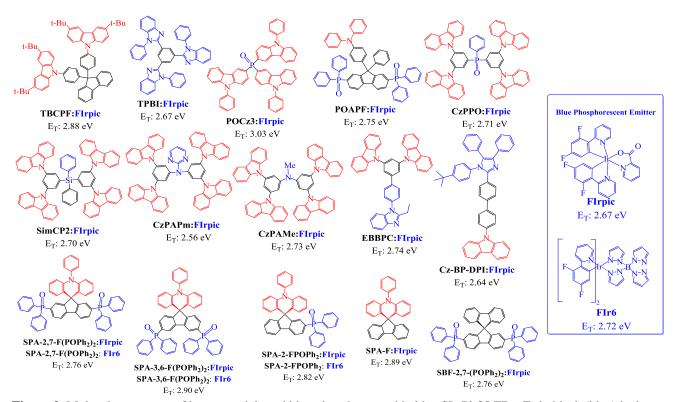
**Figure 2.** Molecular structure of host materials and blue phosphors used in blue SL-PhOLEDs.  $E_T$  in black (blue) is that of the host (phosphorescent emitter). In the host materials, black, blue and red fragments respectively point the  $\pi$ -linker, the acceptor and the donor units.
