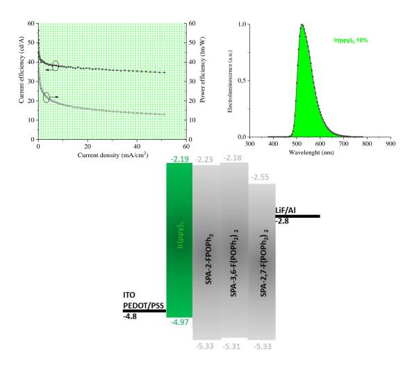
**Figure 8**. Top. Green emitting SL-PhOLED characteristics using as a host **SPA-2,7-F(POPh<sub>2</sub>)<sub>2</sub>** and **Ir(ppy)**<sub>3</sub> as emitter. Left. Current efficiency (cd/A) and power efficiency (lm/W) as a function of the current density (mA/cm<sup>2</sup>). Right. EL spectrum (D53) Bottom. Schematic energy diagrams of the different components used in the EML of green SL-PhOLEDs in the case of SPA-F-POPh<sub>2</sub> family
