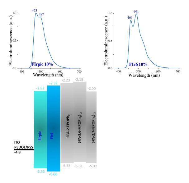
**Figure 5.** Top. Normalized EL spectra of **FIrpic**-based (Left) and **FIr6**-based (Right) SL-PhOLEDs using **SPA-2-FPOPh**<sub>2</sub> as host (D18 and D23). Bottom. Schematic energy diagrams of the different components used in the EML of blue SL-PhOLEDs in the case of SPA-F-POPh<sub>2</sub> family.
