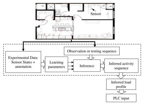
Fig. 1 Plan of a standard home and synoptic of the considered Bottom-Up modeling approach
