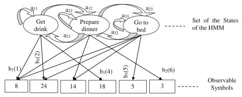
Fig. 5 Graphical representation of a HMM given on an example
