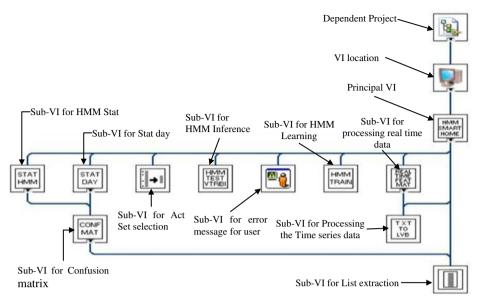
Fig. 3 VI Hierarchy of the principal program showing the main developed sub-VIs icons
