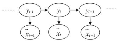
Fig. 6 Interconnection between the sequences of states and the observations of the HMM
