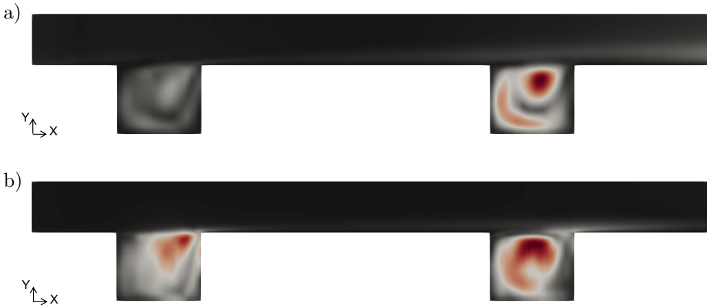
Figure 10: Magnitude of U_{RMS} , comparison and a) 10 m/s and b) 20 m/s.
