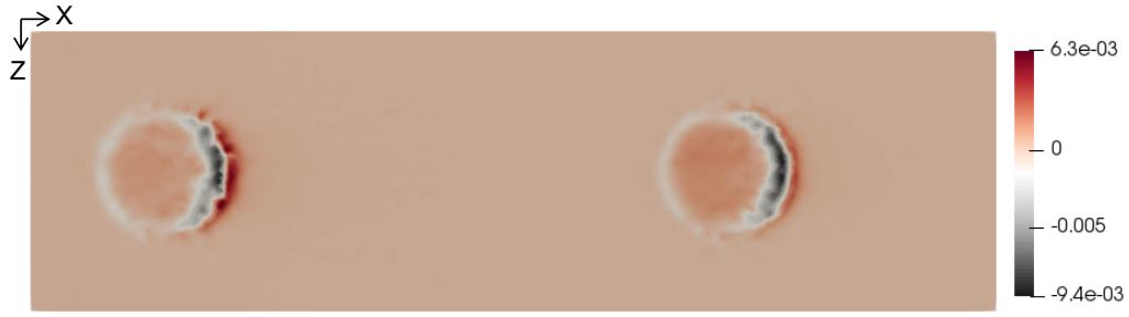
Figure 8: Jetting phenomenon, contour of U_Y/U_\infty at 20 m/s, slice normal to the wall at Y/\delta = 0.01 .
