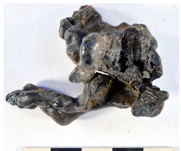
Figure 18. Cord-like slag with charcoal imprints (MWS2002.08); (cl. N. Dieudonné-Glad, HeRMA, Université de Poitiers).
