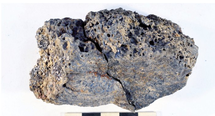
Figure 13. Solid slag with spherical voids on the upper surface (MWS2006.04); (cl. N. Dieudonné-Glad, HeRMA, Université de Poitiers).
