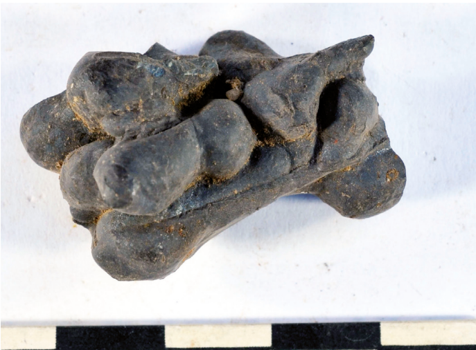
Figure 17. Cord-like slag with only one broken end (MWS2002.13); (cl. N. Dieudonné-Glad, HeRMA, Université de Poitiers).
