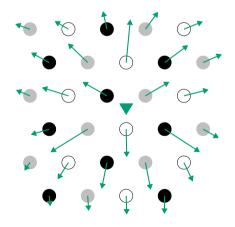
**Figure 8.** Atomic displacements in the (111) plane perpendicular to the dislocation line induced in BCC tungsten by the core dilatation of a screw dislocation in its easy core configuration. Displacement vectors have been magnified by a factor 50. The dislocation position is indicated by a downward triangle.
