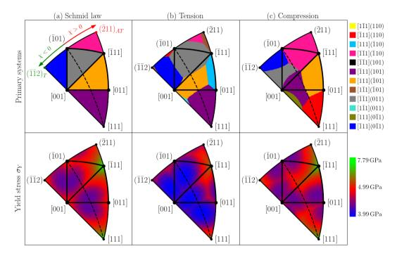
**Figure 13.** Primary  $\langle 111 \rangle \langle 110 \rangle$  slip system (first row) and corresponding yield stress (second row) activated in tungsten single crystals under uniaxial loading at 0 K as a function of the orientation of the deformation axis and predicted using the Schmid law (a), and the yield criterion developed in this work in tension (b) and compression (c). The color coding of the different slip systems and the stress range are indicated in the legend on the left.
