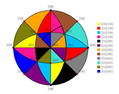
**Figure 12.** Stereographic projection of the BCC lattice showing in colors the regions where each individual  $\langle 111 \rangle \{110\}$  slip system has the highest Schmid factor. The thick black triangle is the minimum irreducible zone of the  $[111](\overline{1}01)$  slip system with  $\zeta \in [0,90^{\circ}]$  and  $\chi \in [-30^{\circ}, 30^{\circ}]$ .
