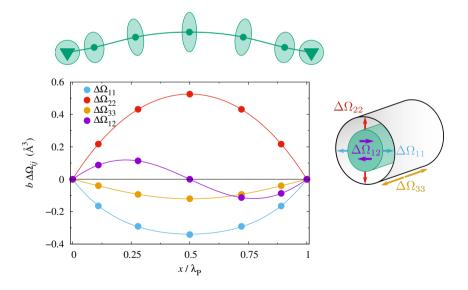
**Figure 9.** Variation of the relaxation volume tensor along the minimum energy path between easy core configurations. The different tensor components are shown as a function of the dislocation position *x* along the glide direction normalized by the distance  $\lambda_P$  between Peierls valleys. The corresponding shape of the 2D Eshelby inclusion along this path is sketched in the upper part.
