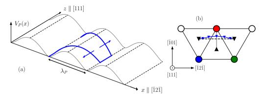
**Figure 16.** (a) Sketch of a dislocation line (blue) crossing a Peierls barrier through the nucleation and propagation of a kink pair. (b) Projection of the 1/2[111] screw dislocation trajectory gliding in the ( $\overline{101}$ ) plane with the three most displaced [111] atomic columns represented in blue, red and green.
