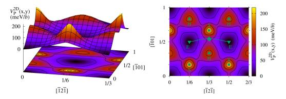
**Figure 4.** 2D Peierls potential of the  $1/2 \langle 111 \rangle$  screw dislocation in BCC tungsten [43]. In the projection on the right, the dislocation trajectory corresponding to the minimum energy path between two easy cores (Fig. 3a) is shown with a green solid line, while the dashed green line links the split and the hard cores (energy variation shown on Fig. 3b). The green diamond corresponds to the saddle configuration.
