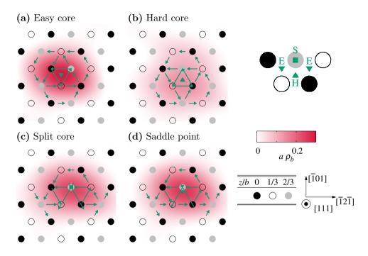
**Figure 2.** Core structures of a screw dislocation in BCC tungsten [21, 43]: (a) easy, (b) hard, (c) split cores, and (d) saddle configuration. The centers of the dislocation are indicated by colored symbols and are sketched in the right panel. Differential displacements and Nye tensors are shown as in Fig. 1.
