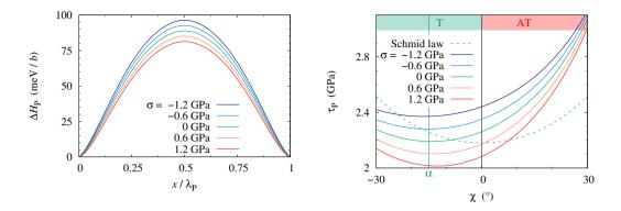
**Figure 10.** Dependence of the Peierls enthalpy barrier (left) and yield stress (right) on a non-glide stress  $\sigma$  perpendicular to the MRSSP (*cf* Eq. 16 for the stress tensor definition).  $\chi$  is the angle between the MRSSP and the {110} glide plane and is null in the left figure.
