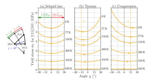
**Figure 19.** Yield stress of the  $[111](\overline{101})$  slip system predicted from Eq. 28 at different temperatures as a function of the angle  $\chi$  for  $\zeta = 45^{\circ}$ : according to Schmid's law (a) and including non-Schmid effects in tension (b) and compression (c). The angle  $\chi$  leading to a minimum yield stress is indicated by a square symbol. Parameters as in Fig. 18
