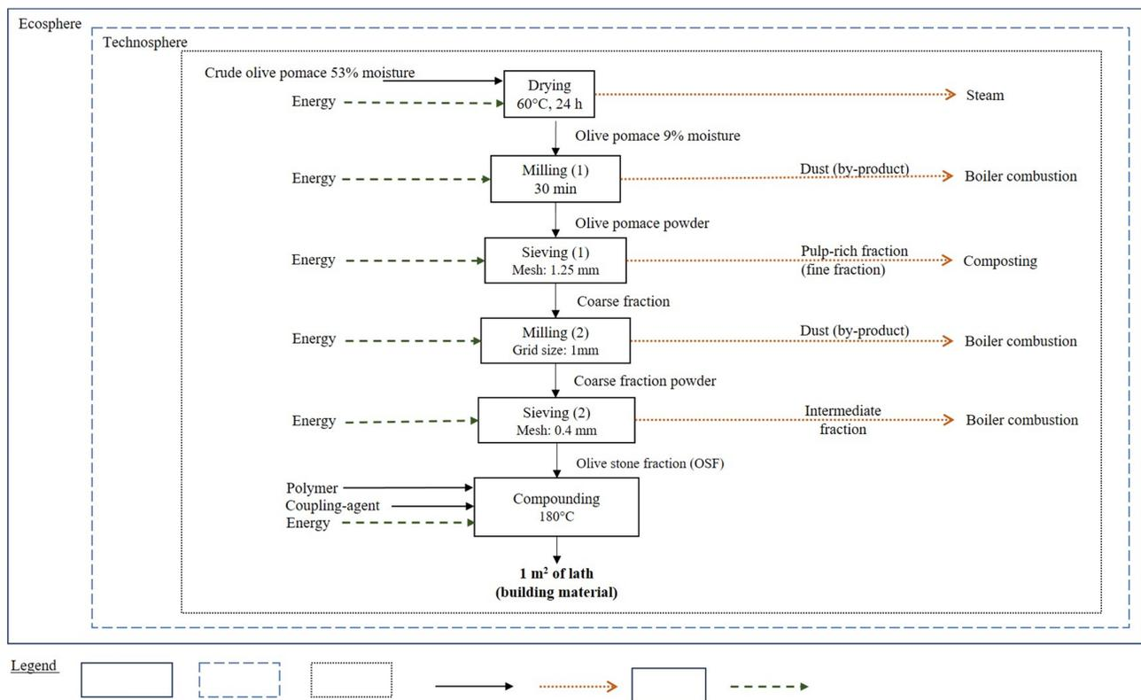
**Figure 3.** Process tree of the olive pomace-based composite.
