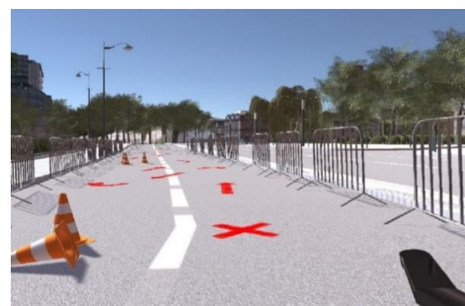
Figure 3. Participant point-of-view during trials. The black part in the bottom-right corner corresponds to the arm of a virtual wheelchair, which is spatially co-located with the real joystick and vestibular feedback platform.
