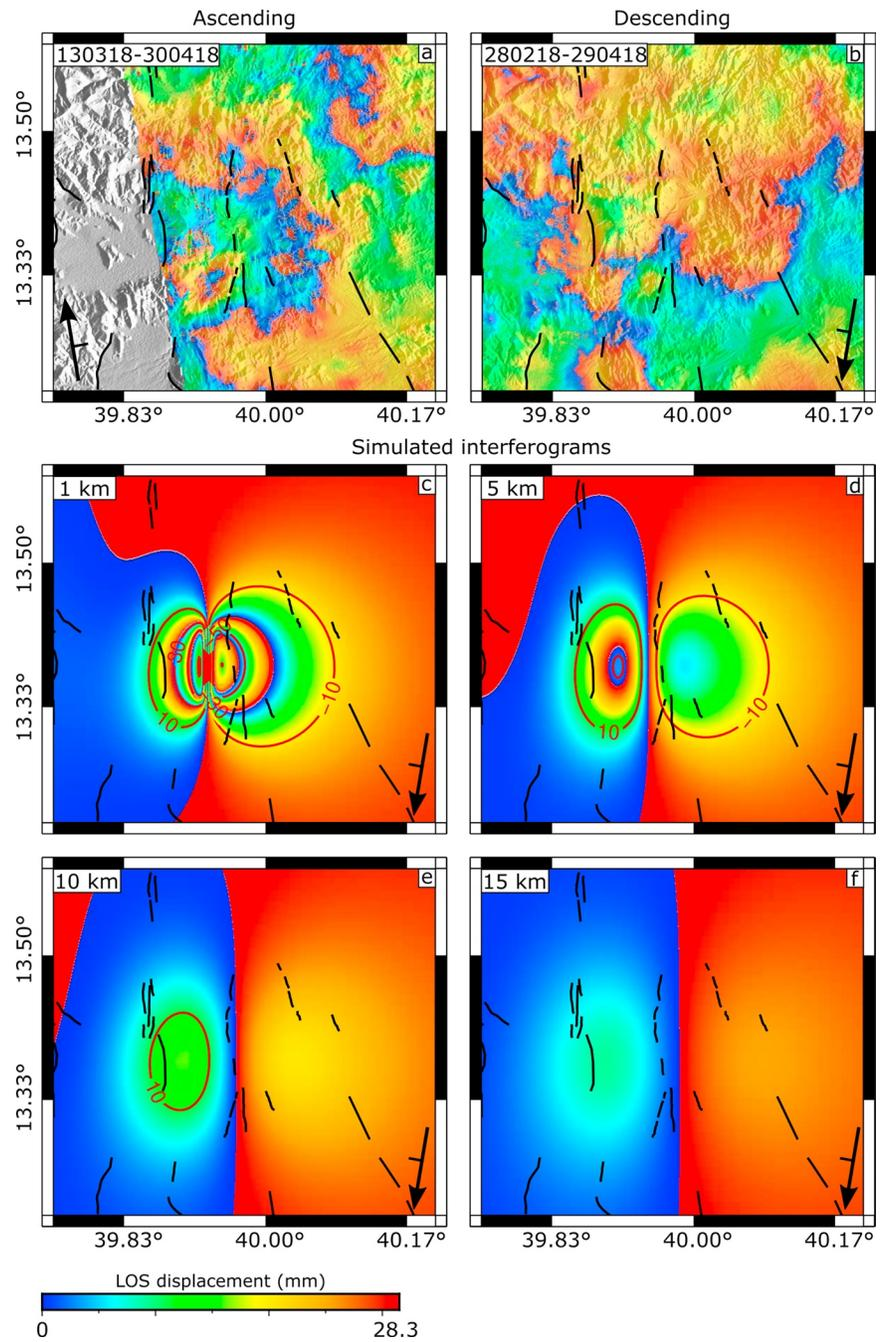
**Figure 5.** (a and b) Measured wrapped coseismic interferograms from Sentinel-1 acquisitions. (c-f) Simulated wrapped interferograms assuming Okada shear dislocation model located at increasing depth. The red contour lines display the unwrapped deformation in mm. Black solid lines are faults reported by Zwaan et al. (2020b).
