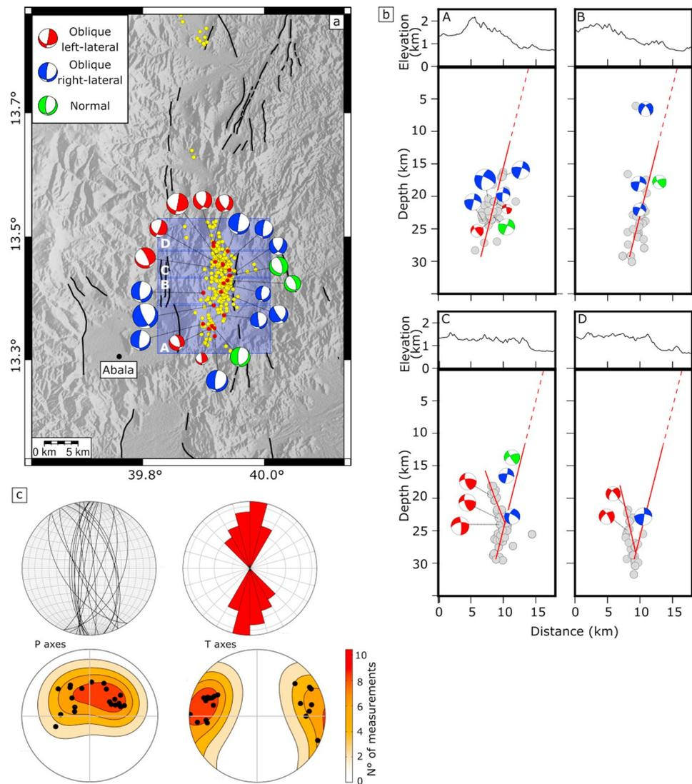
**Figure 4.** Focal mechanism solutions in map view (a) and cross sections (b) for events located with >15 stations. Yellow dots in (a) and gray dots in (b) are the relocated seismicity. Red lines in (b) represents possible faults highlighted by the relocated seismicity. (c) The plots show the stereographic projection of the strike and dip (top left), the rose diagram of the strikes (top right), and the *P* and *T* axes of the main nodal planes with contour of number of measurements (bottom).
