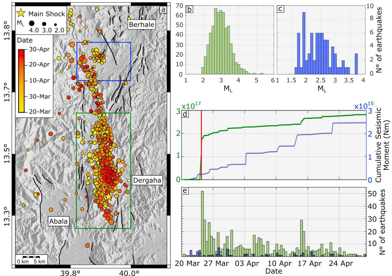
**Figure 3.** (a) Epicentral distribution of the 673 earthquakes located with NLLoc (Lomax, 2000) and occurred between March 20, 2018 and April 30, 2018. The earthquakes are color-coded by time. The blue and green boxes highlight the two marginal grabens along the North-Western Afar Margin (NWAM). (b and c) Histograms of magnitudes for the two areas highlighted in (a). (d and e) Cumulative seismic moment curves and histograms of number of earthquakes for the two areas in (a).
