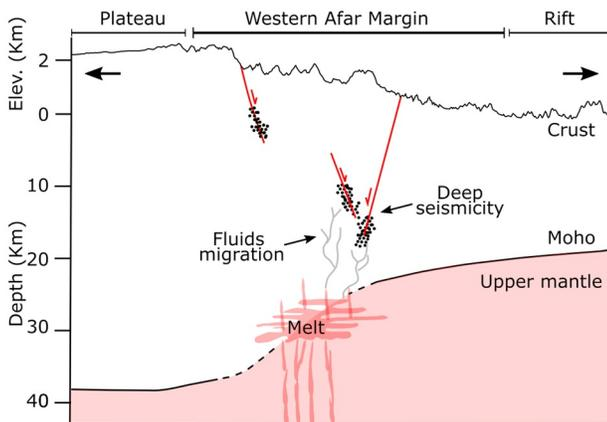
**Figure 6.** Simplified sketch showing the interpretation and proposed mechanism controlling the deep seismicity below the Dergaha graben. We interpret deep seismic activity along rift border faults to be induced by magma migration or the release of fluids such as mantle-derived CO<sub>2</sub>.
