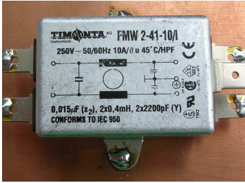
Figure 7. Photograph of under study EMI low-pass filter.
