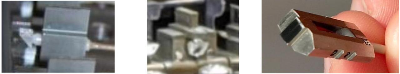
Figure 1. MOS button assembly with its 1.5 mm prism on the test bench (left), mIFU button assembly with its 2 mm prism located under the lens holder on its retractor (center) and MOS slitlet during inspection with its 24 fibres (right).
