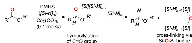
Scheme 5. Plausible mechanism of the formation of Si-O-Si bridges between PMHS chains in presence of carbonyl groups.
