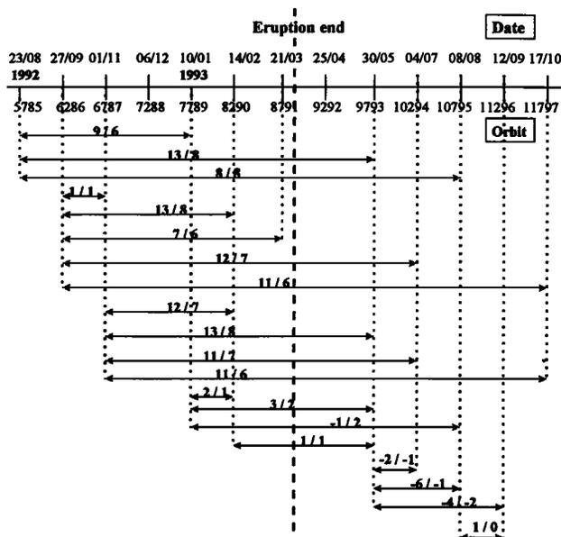
**Figure 3.** Subsidence of the summit of Etna (in cm) observed between 23/08/92 and 17/10/93. First bold number corresponds to maximum displacement observed without tropospheric correction, second one after tropospheric correction. Uncertainty on the results is 3 cm.
