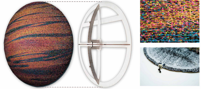
Fig. 18. A complex knitted object showcasing high-level capabilities of the KnitKit system. Custom 5-color stitch templates, action definitions for an integrated drawstring channel and shaping techniques are used to generate the object from a geometric and image texture input. Inset photos show the close-up details of the complex stitch pattern and drawstring channel.
