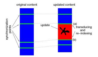
Figure 6: Re-indexing between synchronization points
