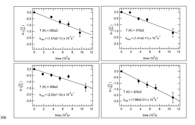
Figure 6 Typical normalized iodine concentration temporal profiles for experiments carried out in the  $283 \le T(K) \le 323$  temperature range and at 40%RH following photolysis of the I<sub>2</sub> adsorbed on SiO<sub>2</sub> particles. The solid lines are obtained from least squares analyses and give the expressions for k<sub>obs</sub> shown in the figure. The quoted uncertainties in the k<sub>observed</sub> values are  $68\% (1\sigma)$  confidence limits from the linear regression fit.
