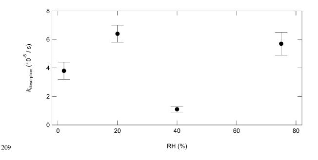
Figure 1 Plot of the obtained first-order rate constants ( $k_{desorption}$ ) for the desorption of iodine as a function of relative humidity. No clear dependence of humidity on the desorption rate constant of I<sub>2</sub> adsorbed on SiO<sub>2</sub> particles is observed. The quoted uncertainties in  $k_{desorption}$ , values are 68% (1  $\sigma$ ) confidence limits from the linear regression fit.
