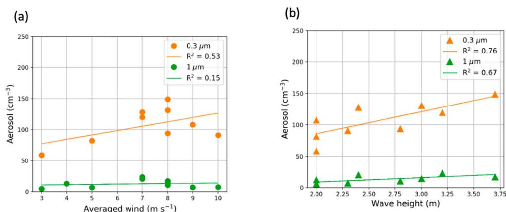
**Figure 16.** Aerosol concentrations (diameter  $>0.3 \mu\text{m}$  and  $>1.0 \mu\text{m}$ ) measured during the BOREAL flights as a function of (a) the averaged horizontal wind in the marine boundary layer and (b) the measured wave height.
