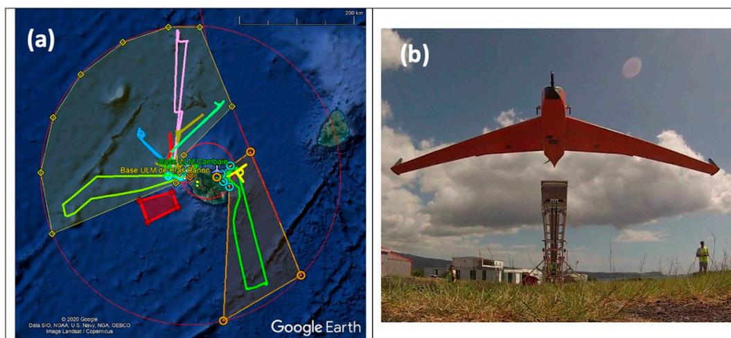
**Figure 15.** (a) The 12 BOREAL flights operated from Réunion Island during the RNR-CYC campaign in February and March 2019. The yellow and orange polygons represent the authorized flight zones to the northwest and southeast of Réunion Island. The outer red circle denotes an operating radius of 250 km around Réunion Island. (b) The BOREAL UAS leaving the catapult for a scientific mission from Cambaie, Réunion Island. Sources: (a) Google Earth; (b) Greg Roberts.
