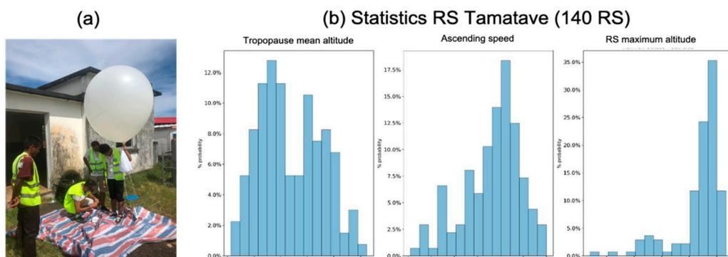
**Figure 3.** The Toamasina (Madagascar) radiosounding campaign. (a) Training of students from Antananarivo University at Toamasina airport. (b) Statistical analysis of the 140 RS measurements performed in Toamasina: mean altitude of the tropopause, ascending speed, and maximum RS altitude. Picture: Olivier Bousquet
