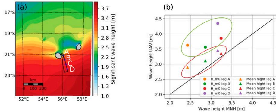
**Figure 19.** (a) WW3 simulation of significant wave height on 29 March 2019 with the BOREAL UAS flight overlaid on the image (black line). The blue crosses correspond to A, B, C and D legs of the flight at 100 m asl. (b) Significant wave height ( $H_{m0}$ ) and mean wave height from the BOREAL UAS observations compared to wave height simulated by WW3.
