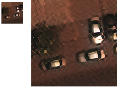
Fig. 6. Example of object reconstruction with super-resolution (factor of 4) of an xView satellite image by SR-WGAN learned from HR aerial images of the Potsdam data.
