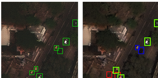
Fig. 8. Detection results from super-resolved image by SR-WGAN (left) and from original image (right).
