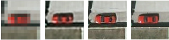
Fig. 4. Super-resolution results obtained by the WGAN compared to SR-IR methods. From left to right: LR image, SR-IR result, SR-WGAN result and HR image.
