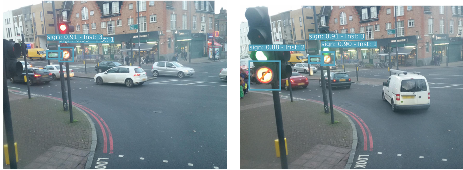
Fig. 4. Sample results obtained on the Mapillary dataset for multi-view object detection and re-identification. Here all detected objects (signs) were both detected and further re-identified (cyan) due to the higher similarity between views.
