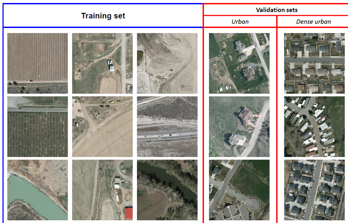
Figure 11. Appearance of new backgrounds in validation sets: the 25-cm VEDAI512 dataset (color version) is divided into three sets: one training set with images acquired in rural, forest, and desert environments; and, two validation sets with new backgrounds from urban and very dense urban areas.
