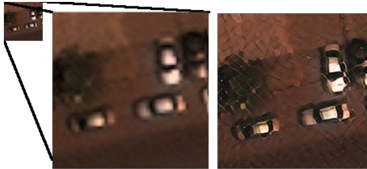
Figure 12. Example of object reconstruction with super-resolution (factor of 4) of an xView satellite image. Left, LR 30-cm xView image zoomed by factor 4; Right: super-resolved image by SR-WGAN learned from HR aerial images of the Potsdam images.
