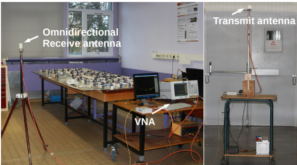
Fig. 2: Practical setup for channel measurements
