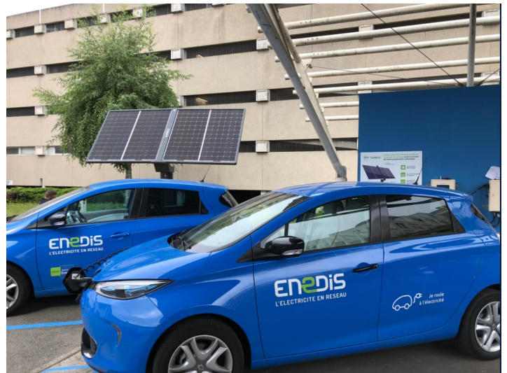
Figure 11: Experimental environment : part of the EVs, EVSEs and PV panels used for our study
